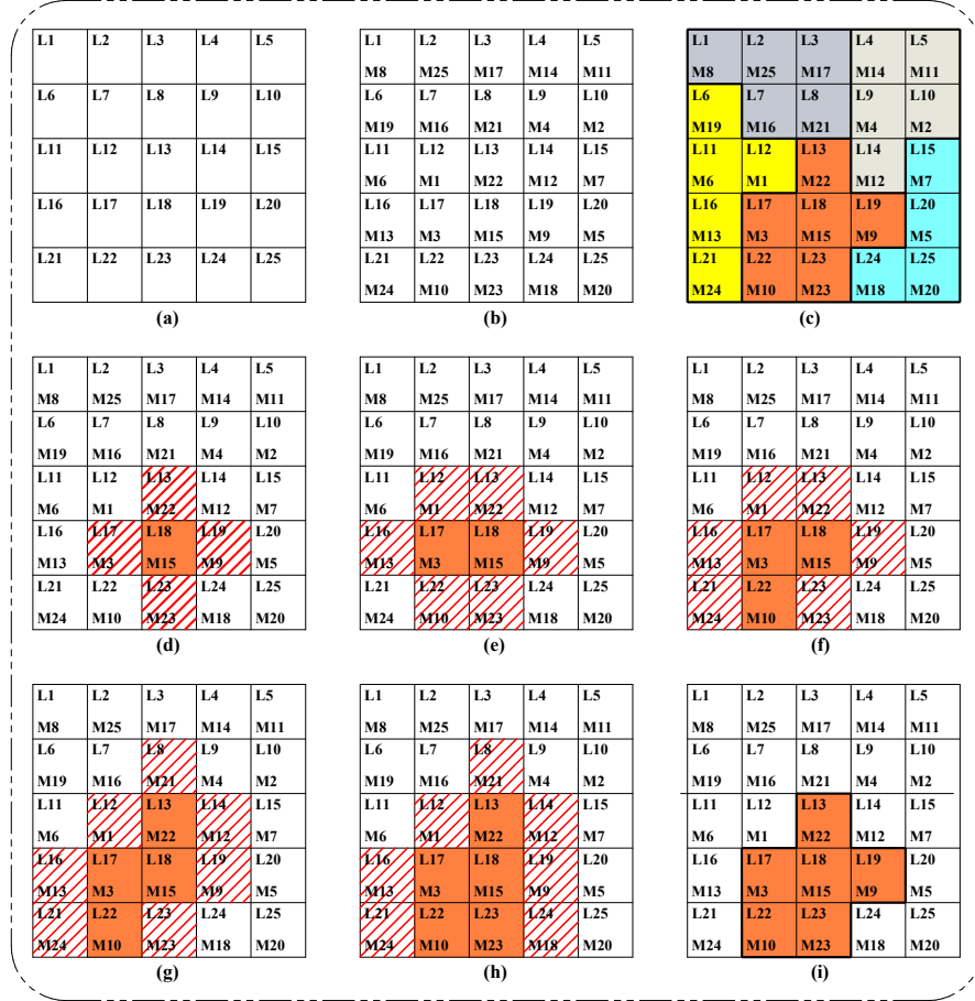
Figure 1: A typical machine distribution and a cell formation process based on location adjacency
